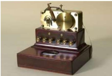
The basic principle of the Wheatstone transmitter was still alive up to the middle of the 19th century. Companies like G.N.T. (Denmark) used it. The photo shows one of its popular transmitters.
