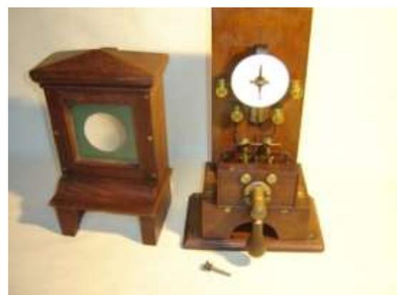
The five photos below show models that were in use as railway signalling instruments.
