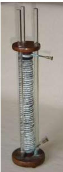
\*Around the year 1800 **Allessandro Volta** (1745-1827) noticed that he could generate an electric current by bringing two different metals into contact with one another. Further research resulted in the ‘voltaic pile’, which comprised a stack of discs in the recurring sequence of copper, zinc and felt soaked in sulphuric acid. That was the start of the development of further research for continuous current sources: the batteries.
