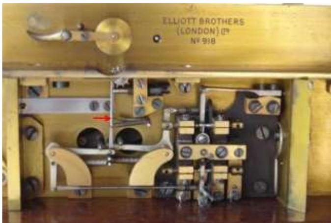
tape is drawn through a paper tape reader (the *transmitter*), by the central line of holes, one hole-spacing at a time. At each position two light metal rods are pressed successively against the paper. The rods operate contacts whenever they pass through a hole, producing positive and negative pulses respectively. When a dot is read two pulses occur in quick succession. When a dash is read their
