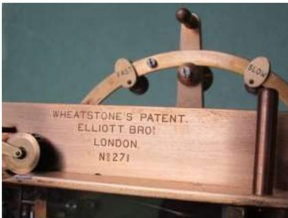
Both the transmitter and the receiver have a speed regulator: see the bow on top of them and the marks SLOW and FAST.
