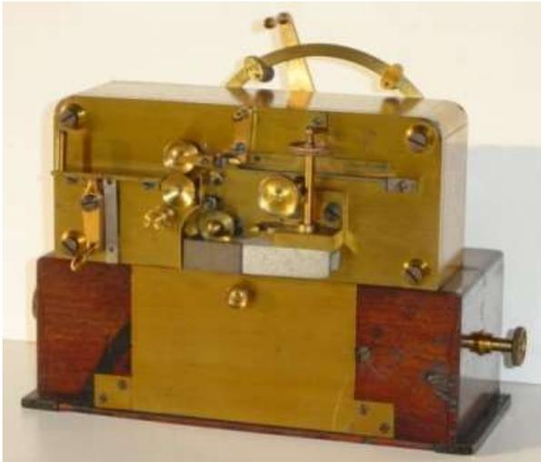
The *receiver* is a sophisticated Morse writer. The dot and dash signals are printed in ink. In the early days, both the transmitter and receiver were driven by a weight, later by a spring motor, and in the end by an electric motor.
